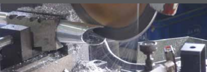
Frame tubes are precisely mitred
