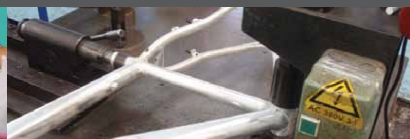
Inspecting frame alignment
