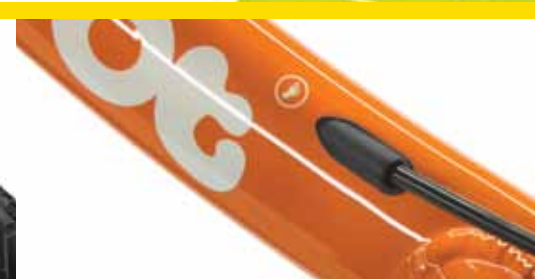
Scoot internal cable routing
