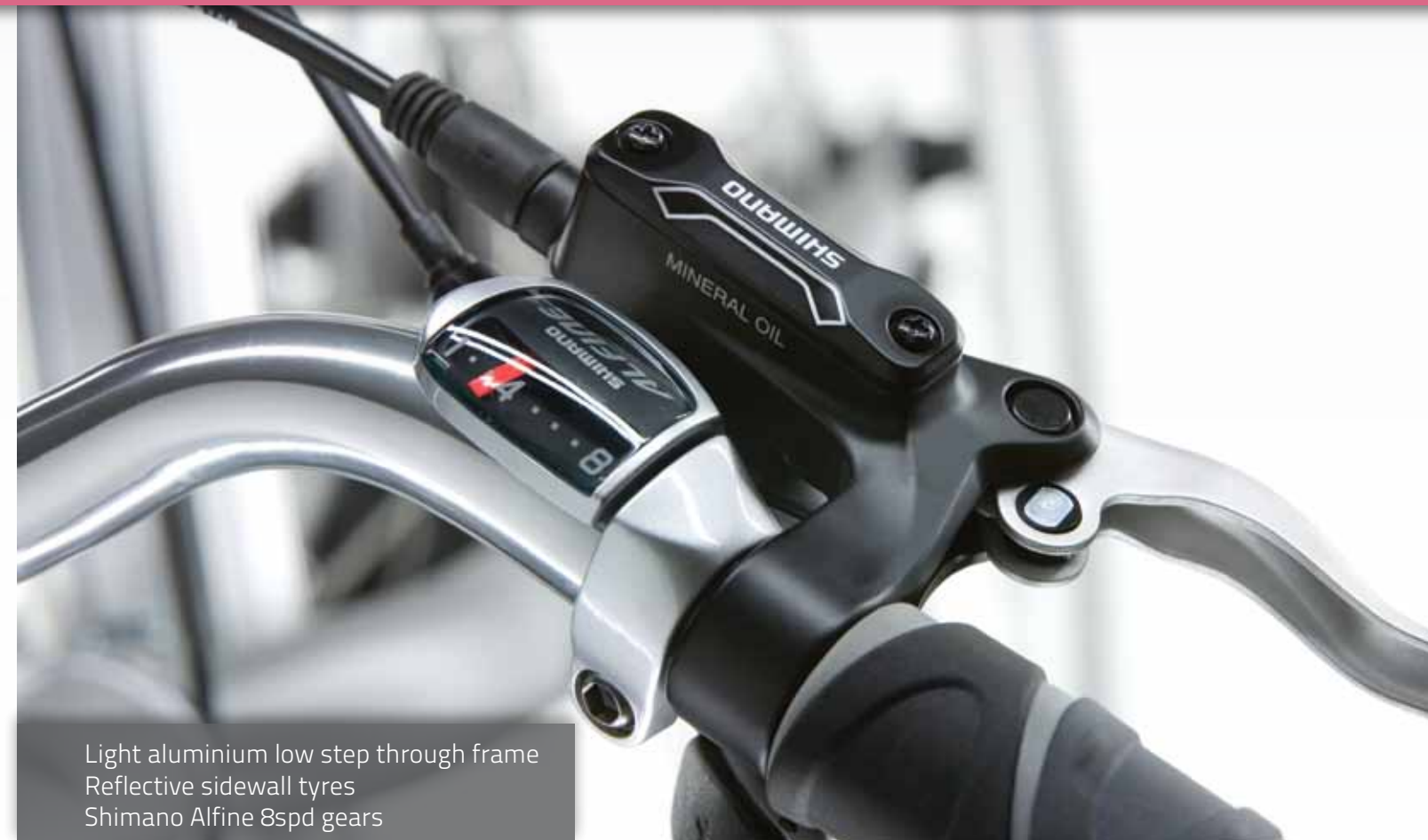
Shimano Alfine for push button shifting
