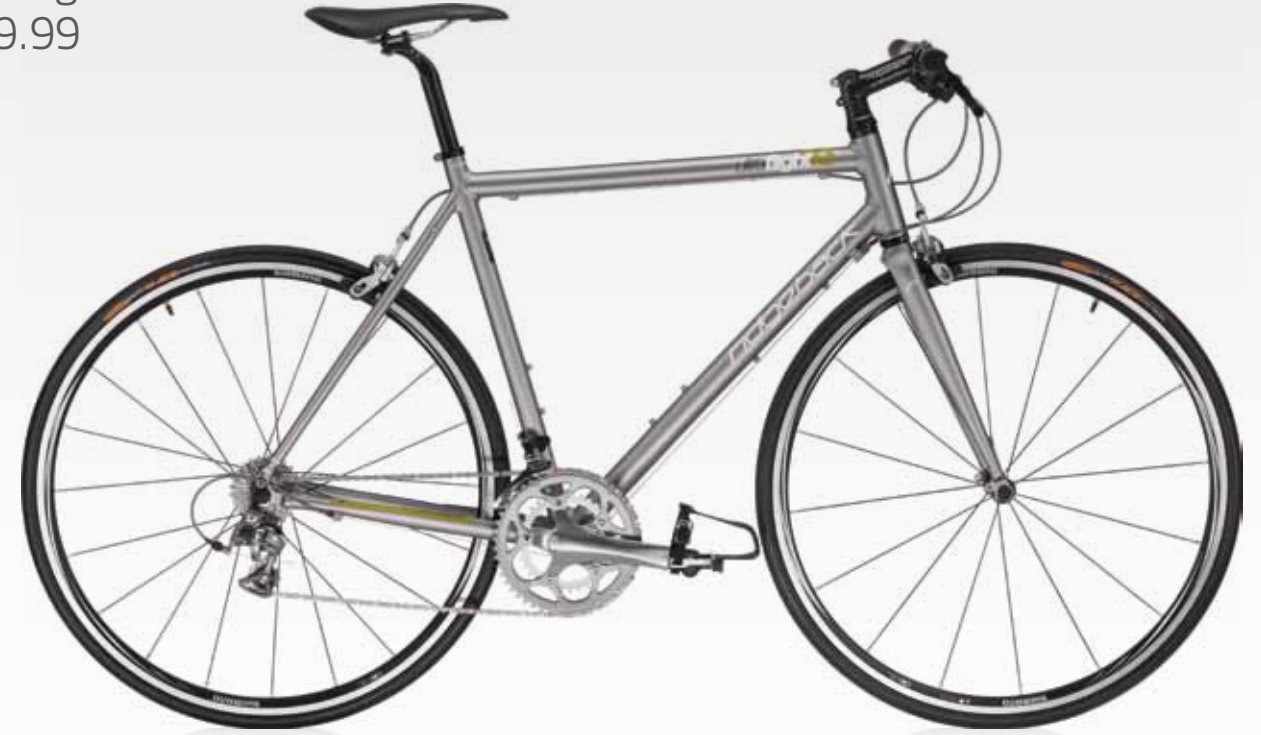
Triple butted frame with Shimano Tiagra 18spd
