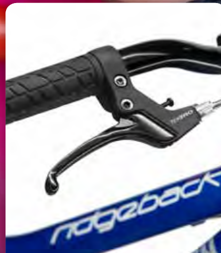
Adjustable reach alloy brake lever
