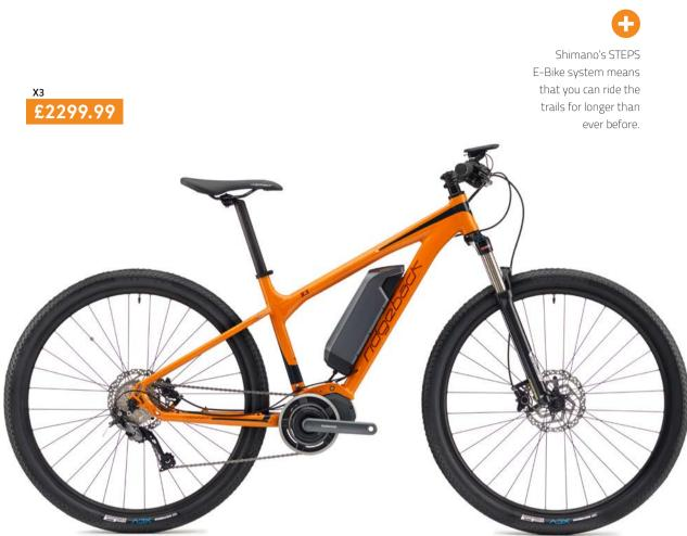
FRAME 6061 heat treated aluminium FORK Suntour XCR-32 LO / 100mm travel SHIFTERS Shimano Altus SL-M370 lever R/H 9 speed CHAINSET Shimano STEPS FC-E6000 / 38T w/CG RIMS Jalco DD28 / 22mm internal / 32h HUBS Shimano RM35 32h / centre lock TYRES Vee Tire Co XCV 29x2.10" MPC BRAKES Shimano BR-M365 / SM-RT10 180mm rotor STEPS Shimano STePS E-6000 / E-6010 head unit / SW-E6000 switch / BT-E6010 battery
