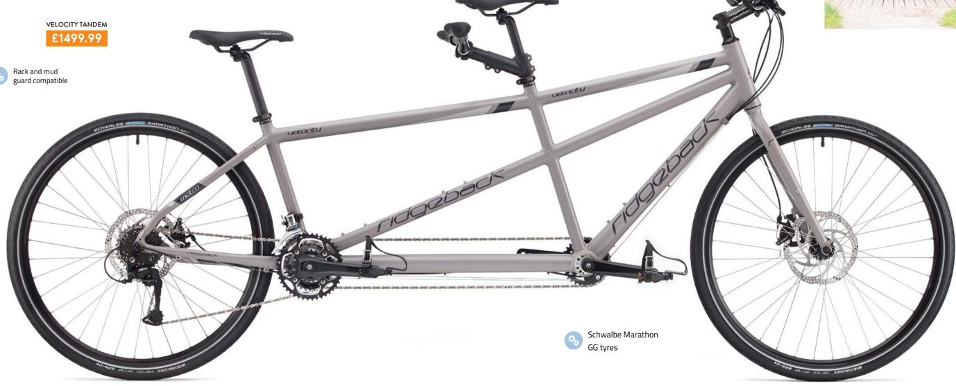
FRAME 6061 heat treated aluminium FORK 6061 heat treated aluminium / mudgaurd eyelets SHIFTERS Shimano ST-EF500 EZ-fire 3x8 speed CHAINSET Lasco TDM-4FM3542 / 44-32-22T / non-drive 32T / 170mm RIMS Wienmann XM-25 Disc / 36h TYRES Schwalbe Marathon GG 700x38c BRAKES TRP Spyke / Tektro TR203-14 203mm
